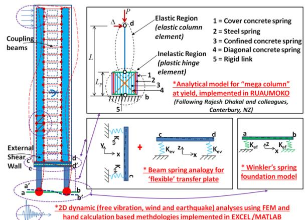
Fig. 2: New approach to modelling a TPHRB
